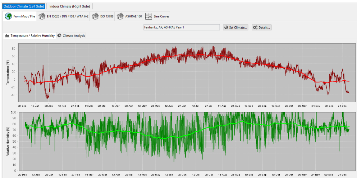
Figure 2: Exterior Climate data used to simulate Fairbanks conditions (wind, solar insolation, and night-sky cooling not shown)
